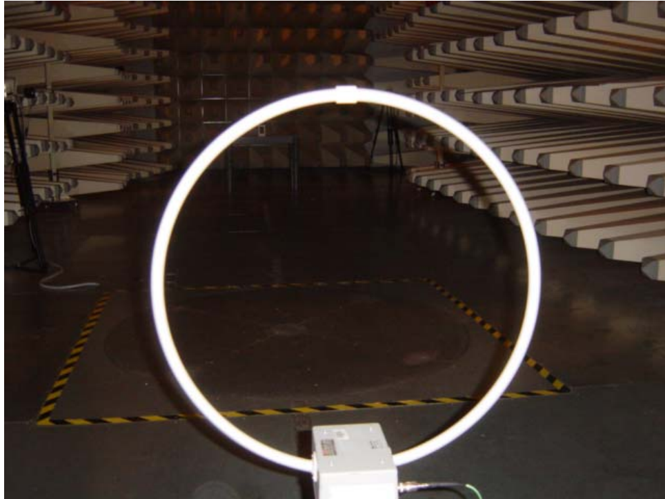
Set up of radiated emission test
