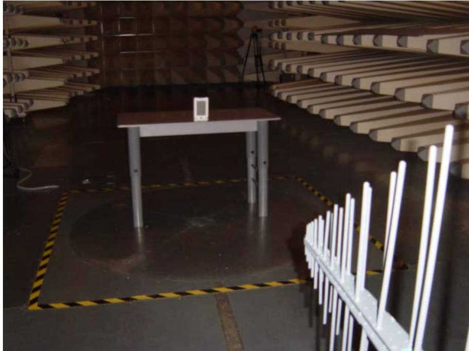
Set up of radiated emission test
