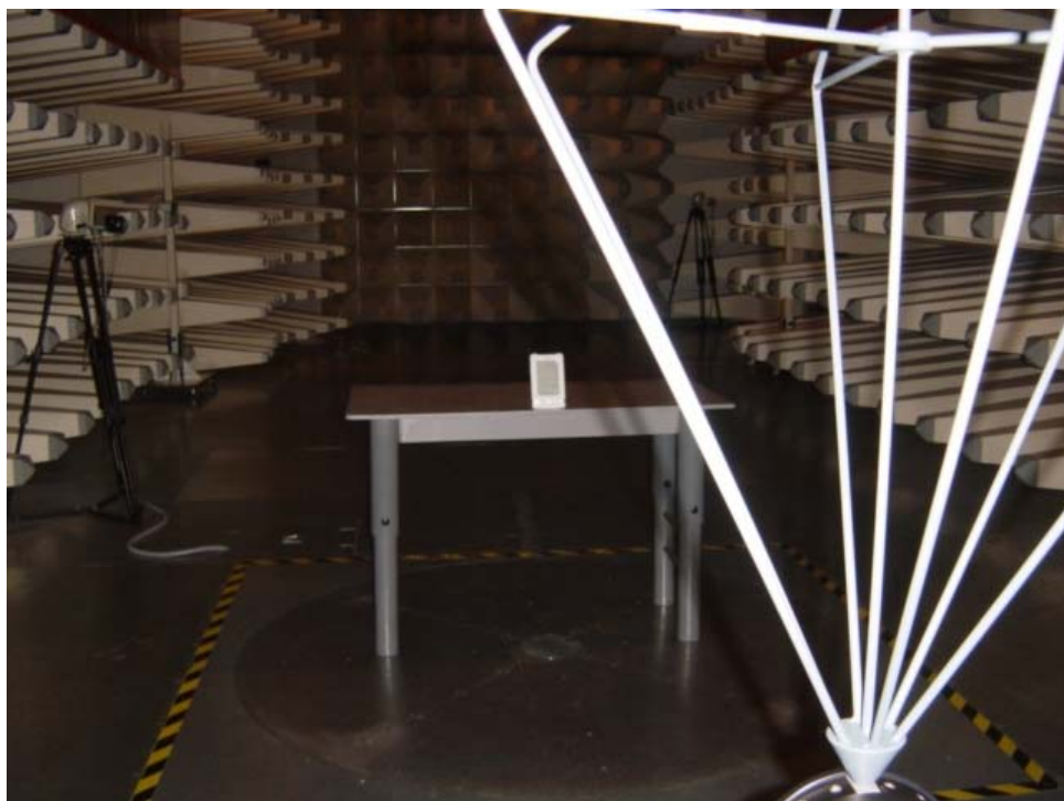
Set up of radiated emission test
