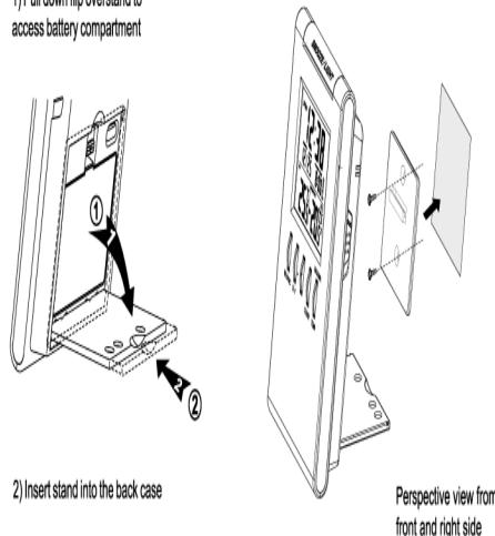
The remote unit comes with a wall mount holder which can hold the unit on wall, or just place it on a flat surface.
