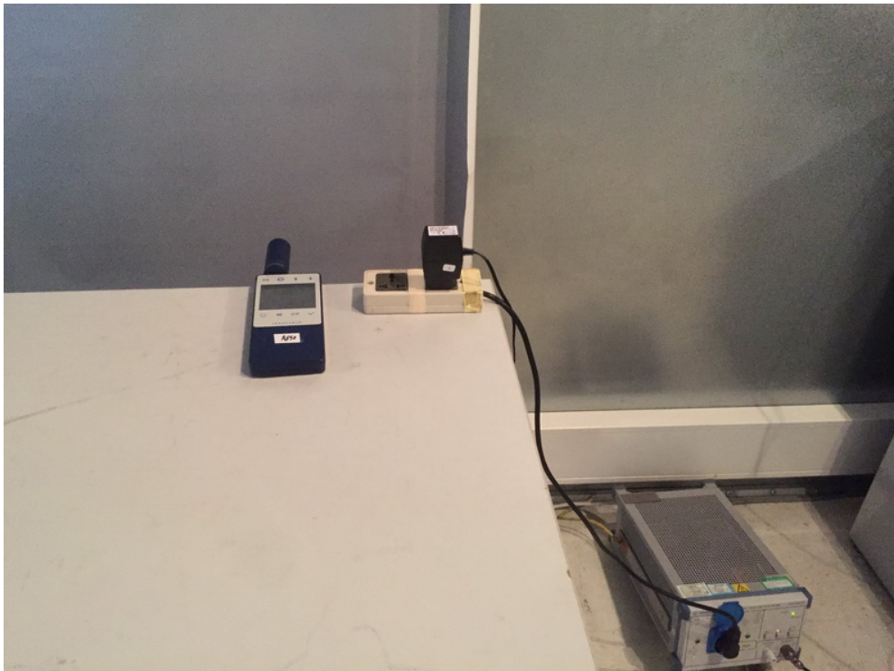
Measurement of Conducted Emission Test Set Up
