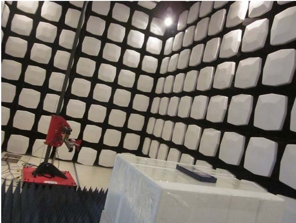
Measurement of Radiated Emission Test Set Up
