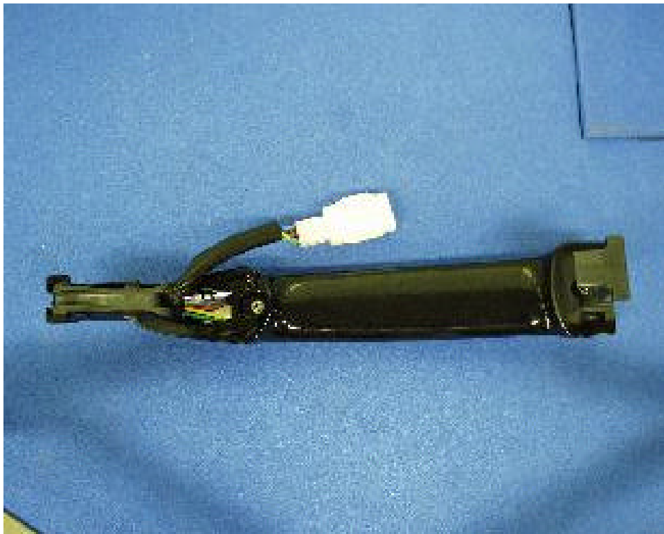
Bottom View of Door Antenna 2(Large)
