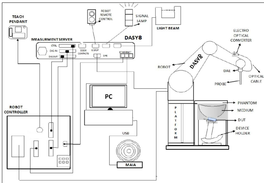
The DASY8 SAR/APD system for performing compliance tests consist of the following items:
