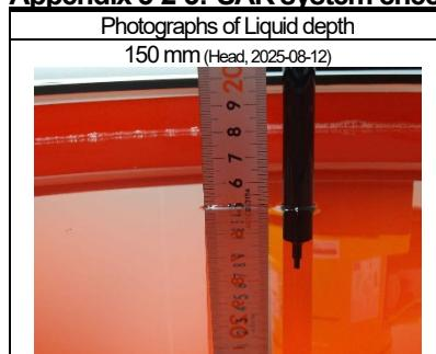
Dipole: CLA-13 - SN1025 ; Mode: CW(0) ; Frequency: 13.000 MHz ; Test Distance: 0 mm (dipole to liquid) ; Power setting: 30.0 dBm
