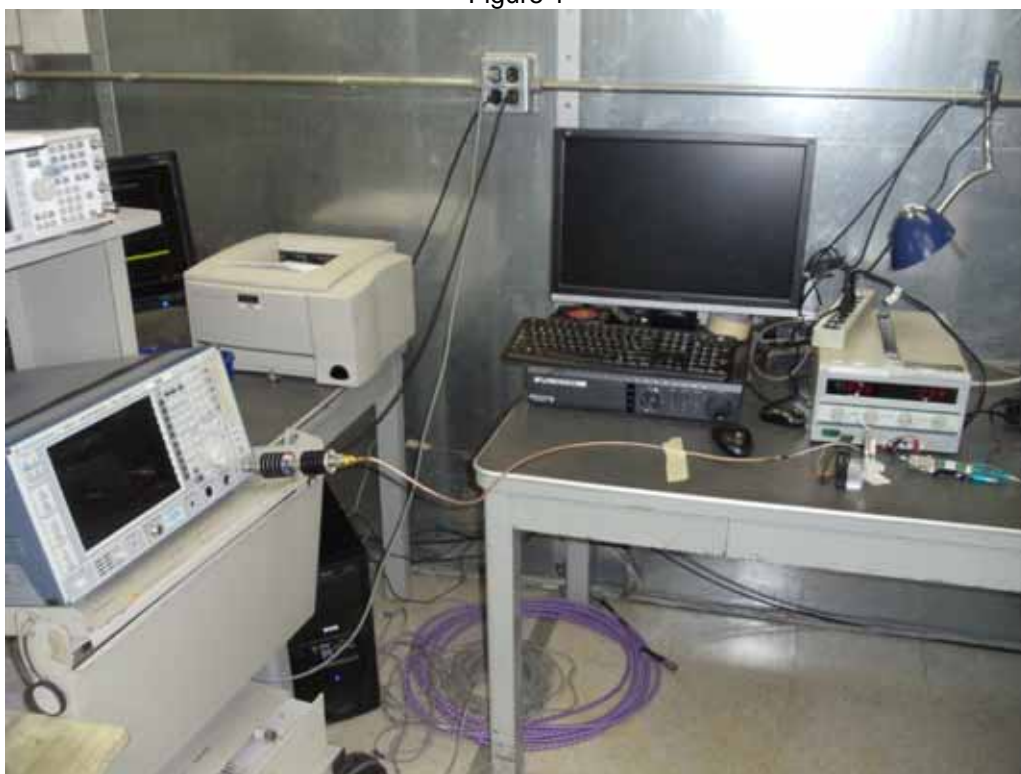
Test Setup for Occupied Bandwidth Emissions FCC Part 101 for the Xeta-9
