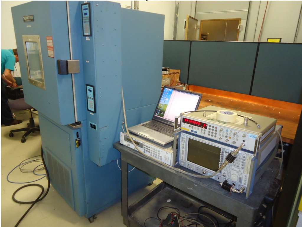
Test Setup for Frequency Stability
