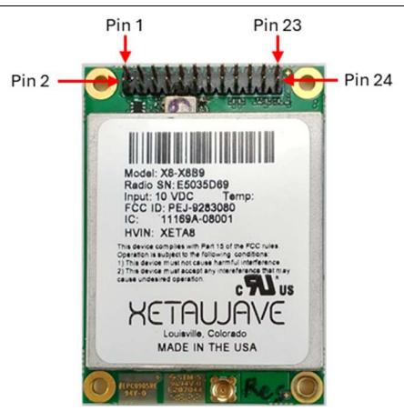
The image shows the Xeta8 radio module with a 24-pin header. The pins are labeled as follows: Pin 1 (top left), Pin 2 (bottom left), Pin 23 (top right), and Pin 24 (bottom right). The module has a barcode and a label with the following text:
