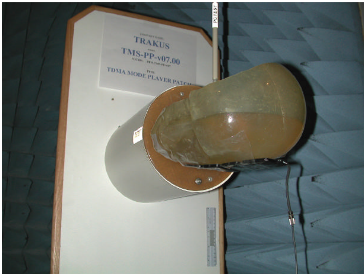
Figure 8. Test Setup of EUT with the source of significant emissions (antenna) 0.2 cm below the phantom.
