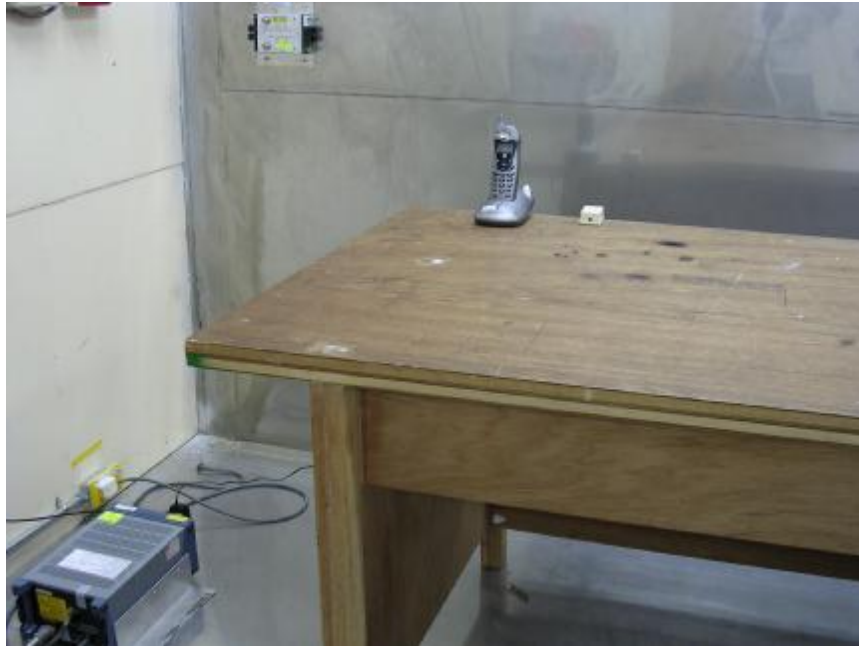
Photo 2: Conducted Emission Test Set-up photo
