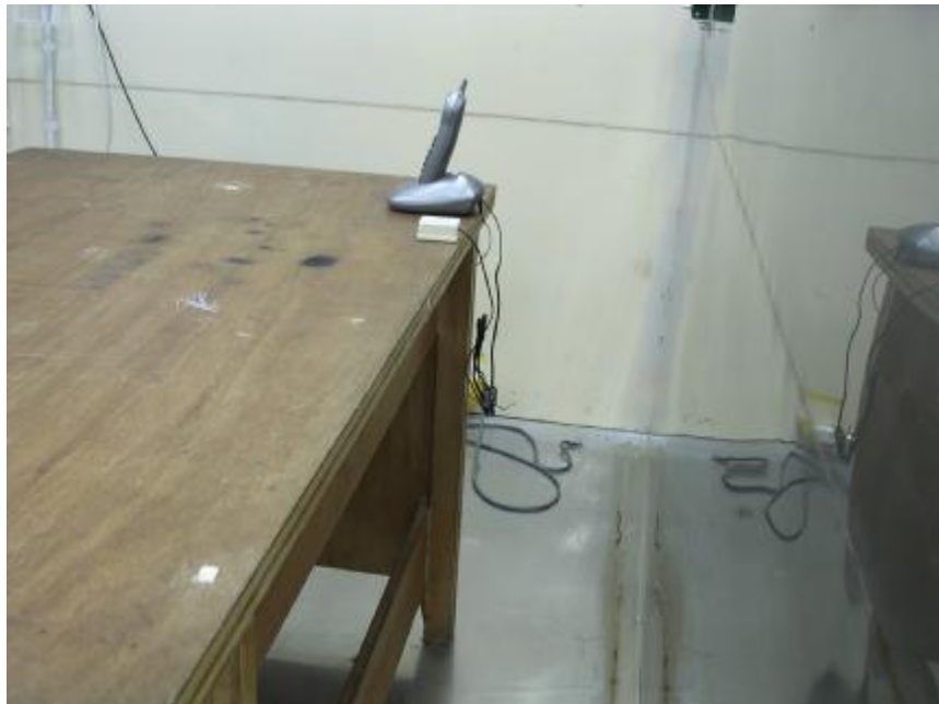
Photo 2: Conducted Emission Test Set-up photo
