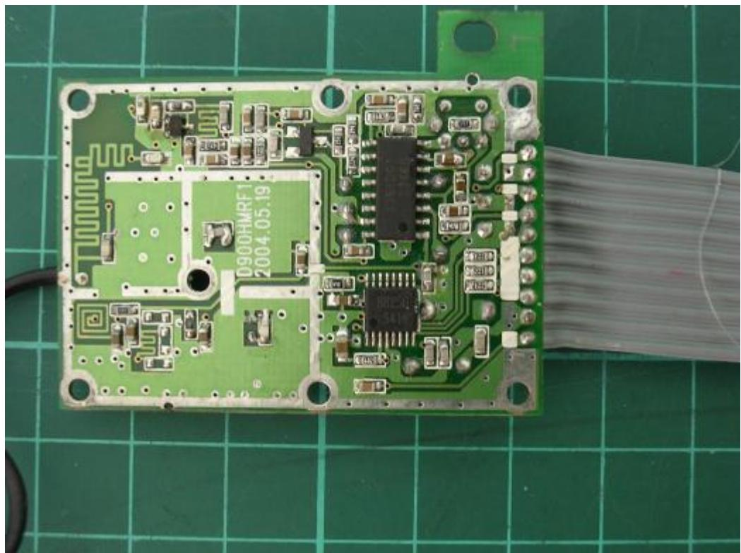
**Photo 20: Internal photo of RF modular (Handset)**
