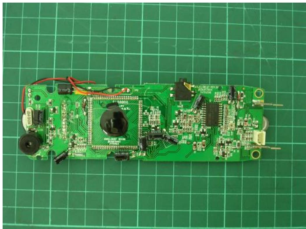
**Photo 16: Internal photo of RF modular (Handset)**
