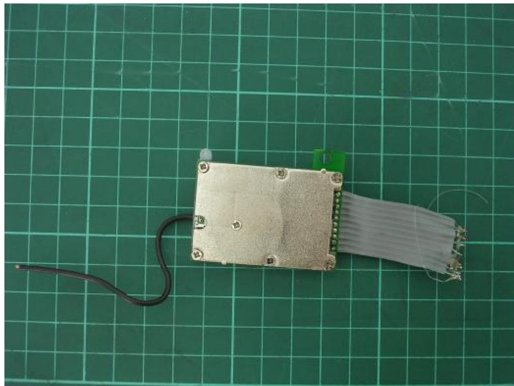
**Photo 19: Internal photo of RF modular (Handset)**
