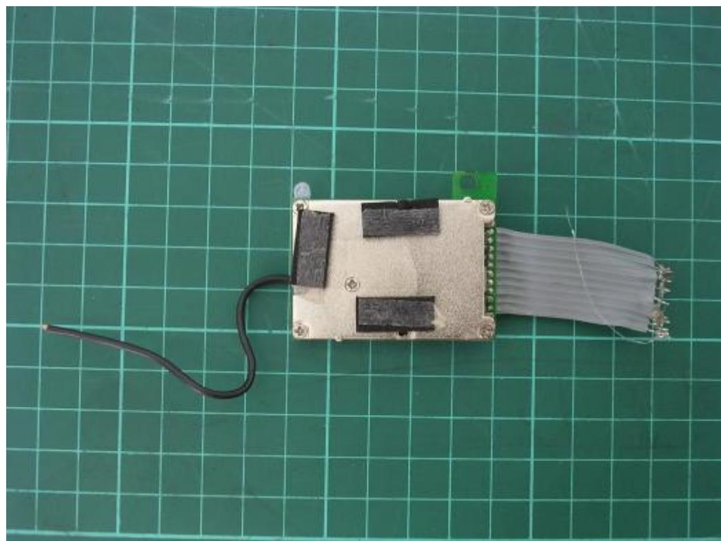
**Photo 18: Internal photo of RF modular (Handset)**
