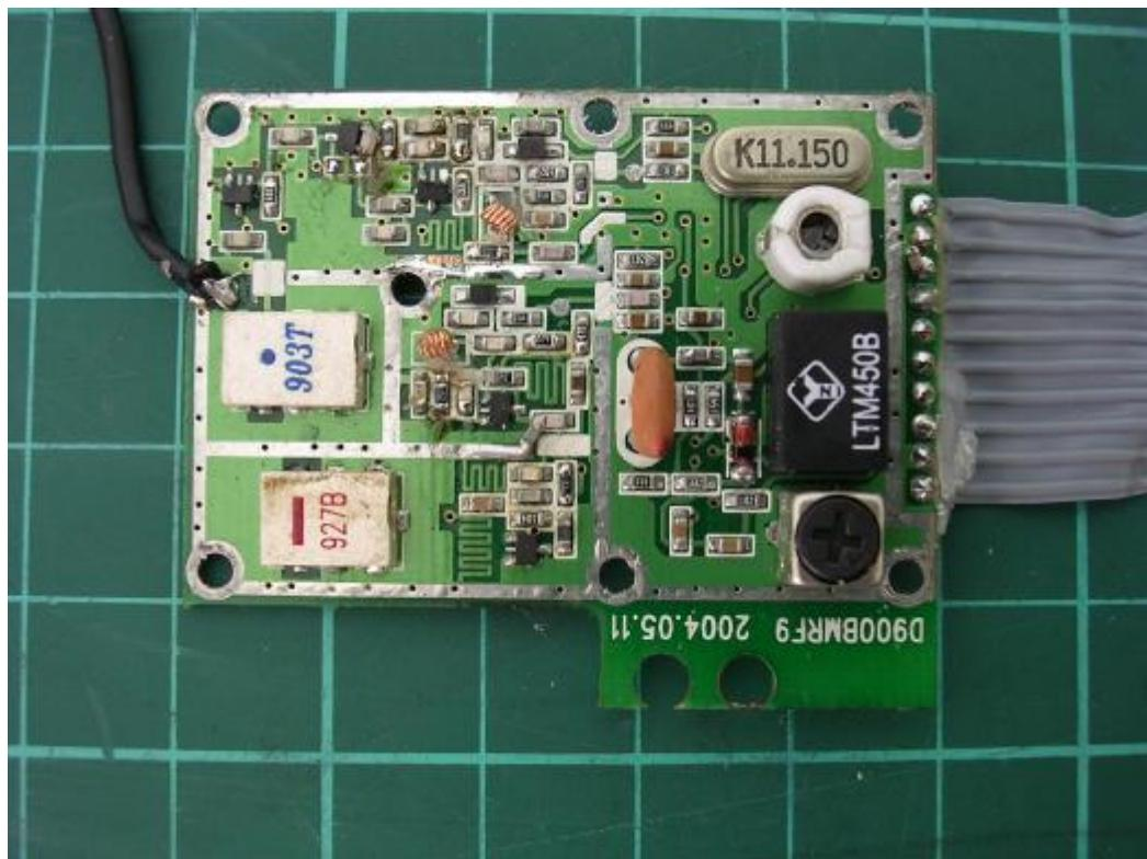
**Photo 11: Internal photo of RF modular (Base)**
