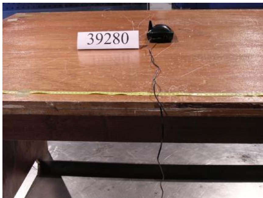
Photo 2: Radiated Emission Test Set-up (Base)
