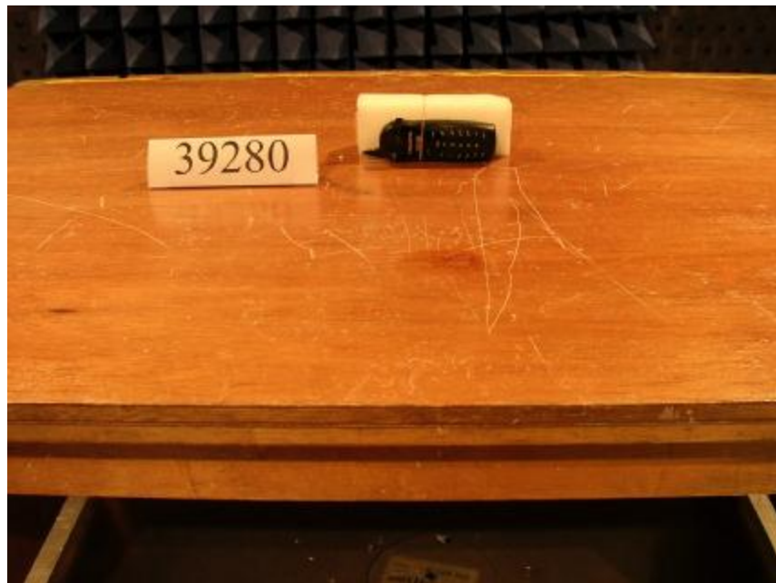
Photo 4: Radiated Emission Test Set-up (Handset)
