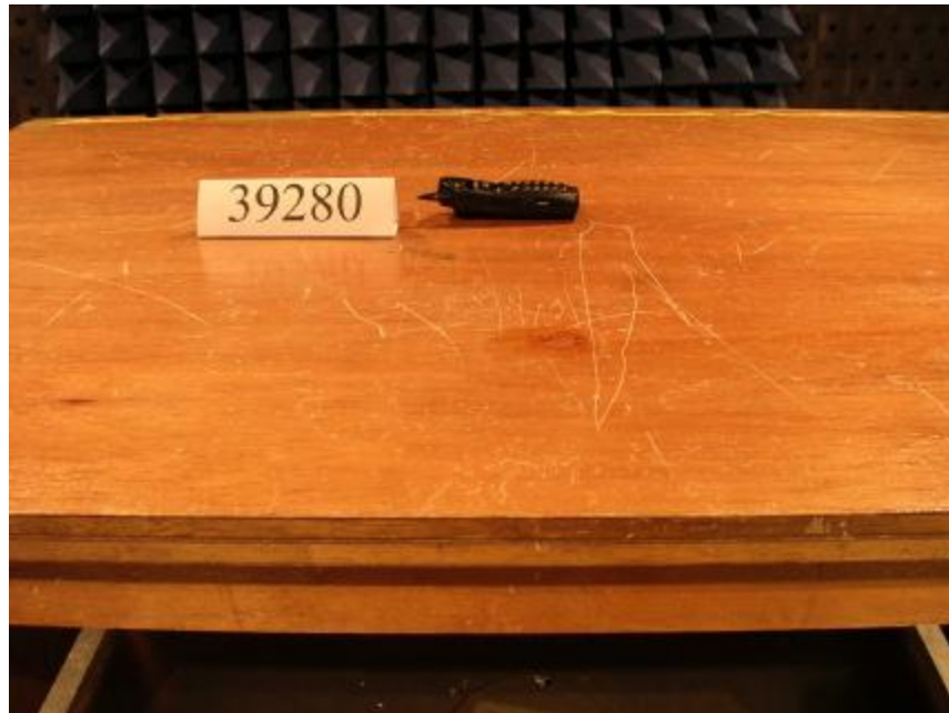
Photo 4: Radiated Emission Test Set-up (Handset)
