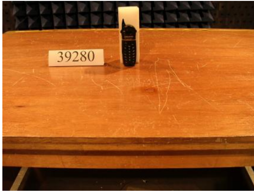
Photo 5: Radiated Emission Test Set-up (Handset)
