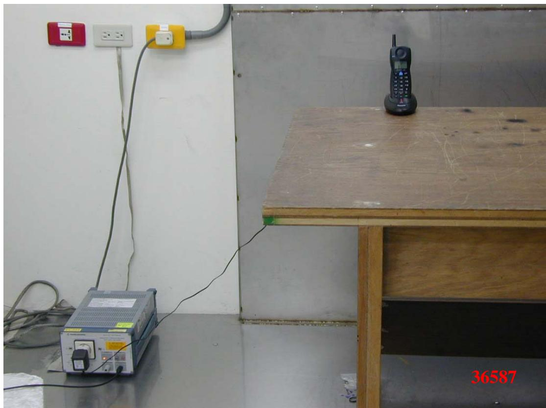
Photo 4: Conducted Emission Test Set-up photo
