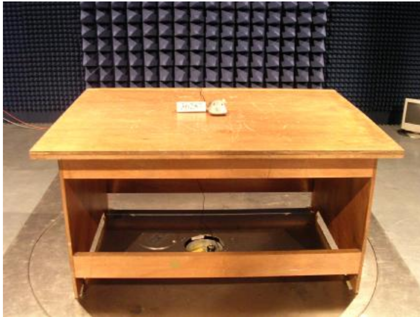
Photo 2: Radiated Emission Test Set-up (Base Unit)
