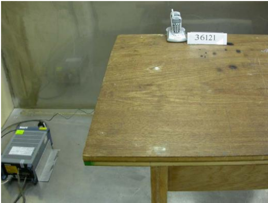
Photo 7: Conducted Emission Test Set-up
