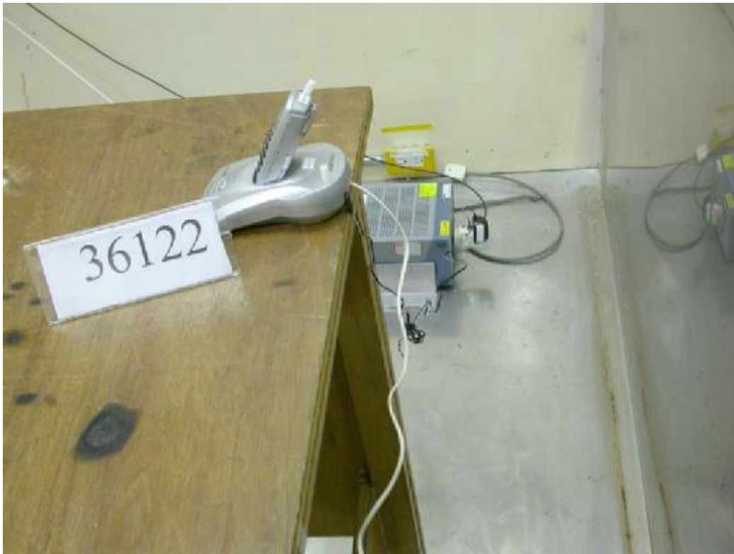
Photo 3: Conducted Emission Test Set-up
