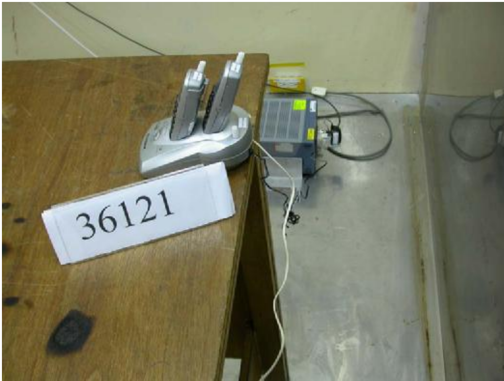
Photo 9: Conducted Emission Test Set-up
