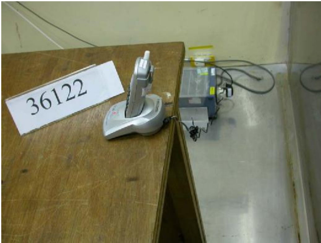
Photo 6: Conducted Emission Test Set-up
