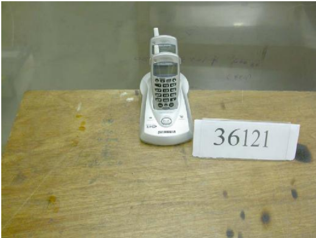
Photo 8: Conducted Emission Test Set-up
