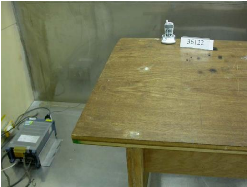
Photo 4: Conducted Emission Test Set-up
