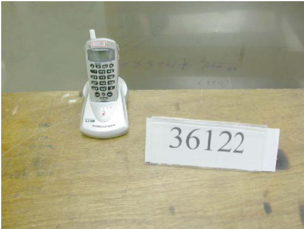
Photo 5: Conducted Emission Test Set-up
