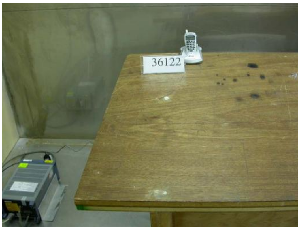
Photo 1: Conducted Emission Test Set-up
