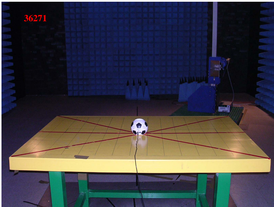
Photo 1: Radiated Emission Test Set-up photo (Base)
