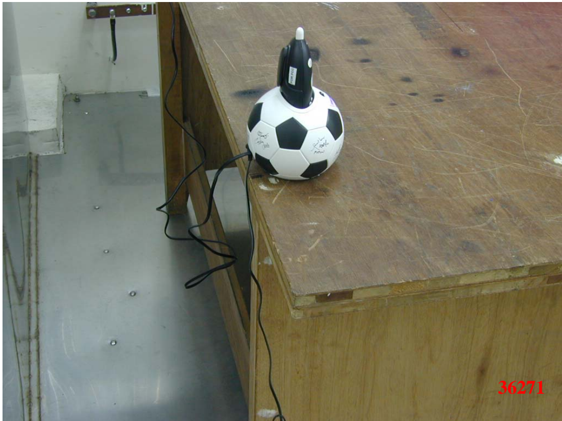
Photo 2: Conducted Emission Test Set-up photo
