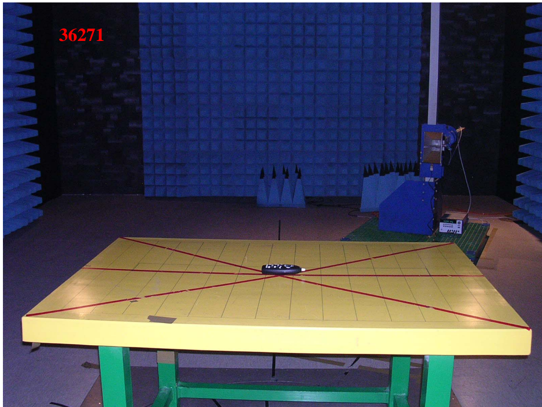
Photo 3: Radiated Emission Test Set-up photo (Handset)
