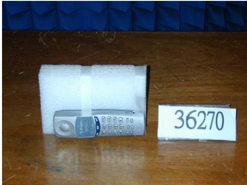
Photo 2: Spurious Test Set-Up photo (Handset)
