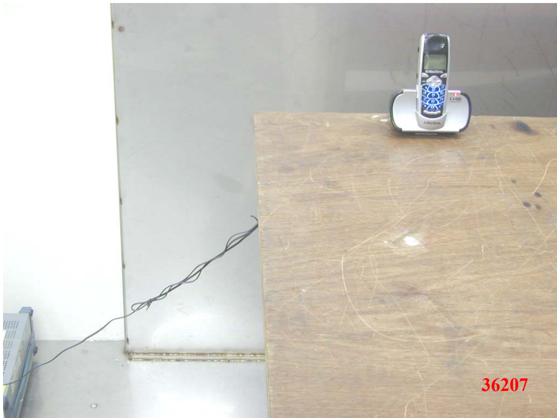
Photo 1: Conducted Emission Test Set-up photo
