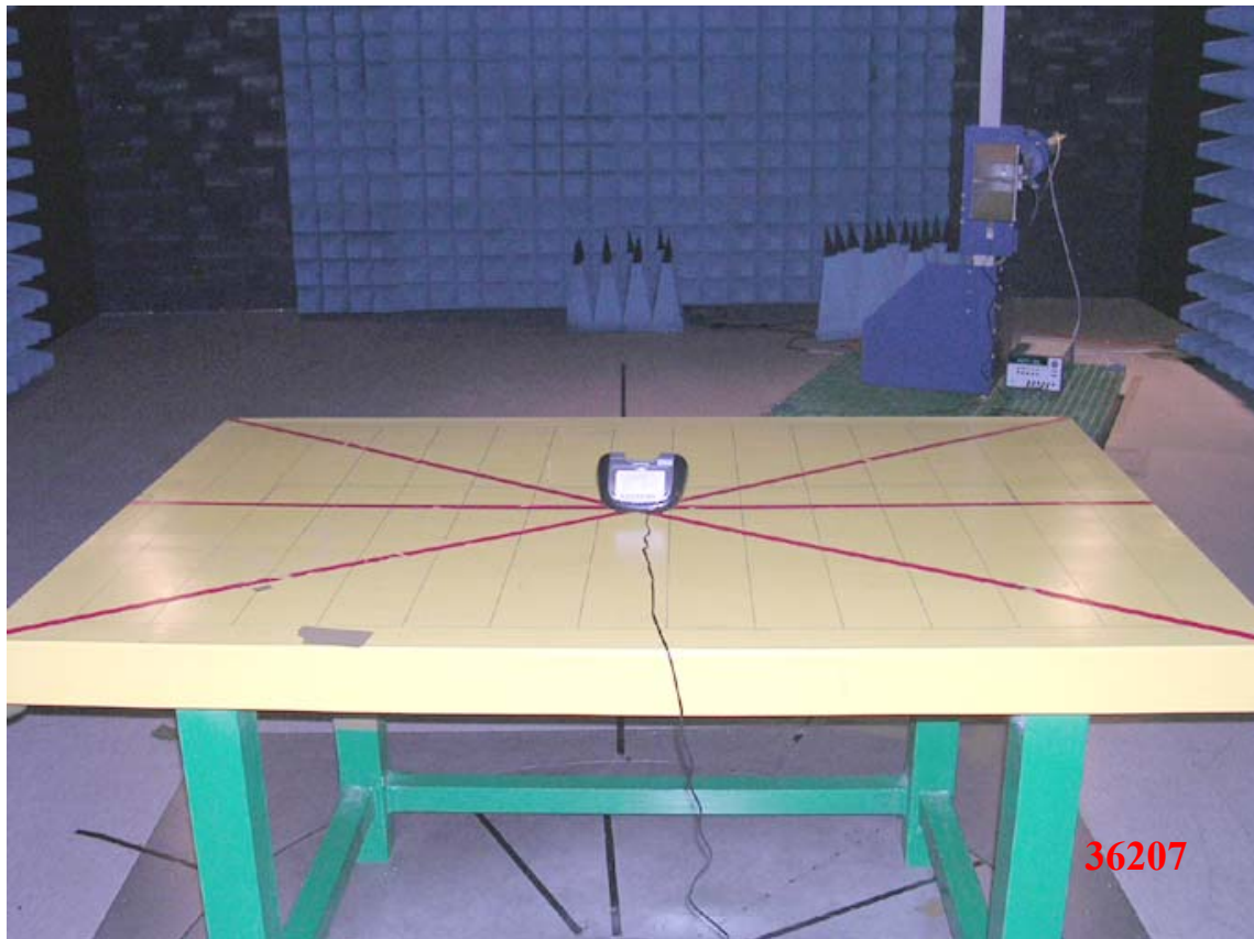
Photo 2: Radiated Emission Test Set-up photo (Base)
