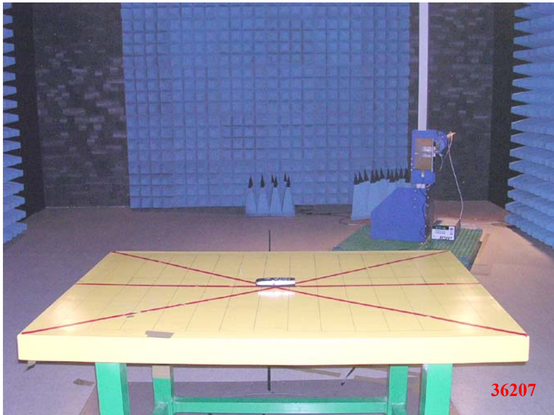
Photo 3: Radiated Emission Test Set-up photo (Handset)
