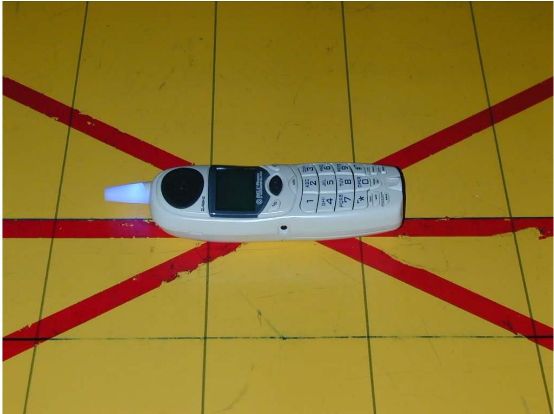
Photo 5: Radiated Emission Test Set-up photo (Handset)
