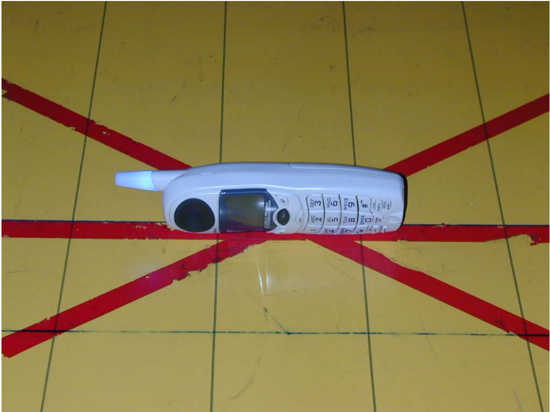
Photo 3: Radiated Emission Test Set-up photo (Handset)
