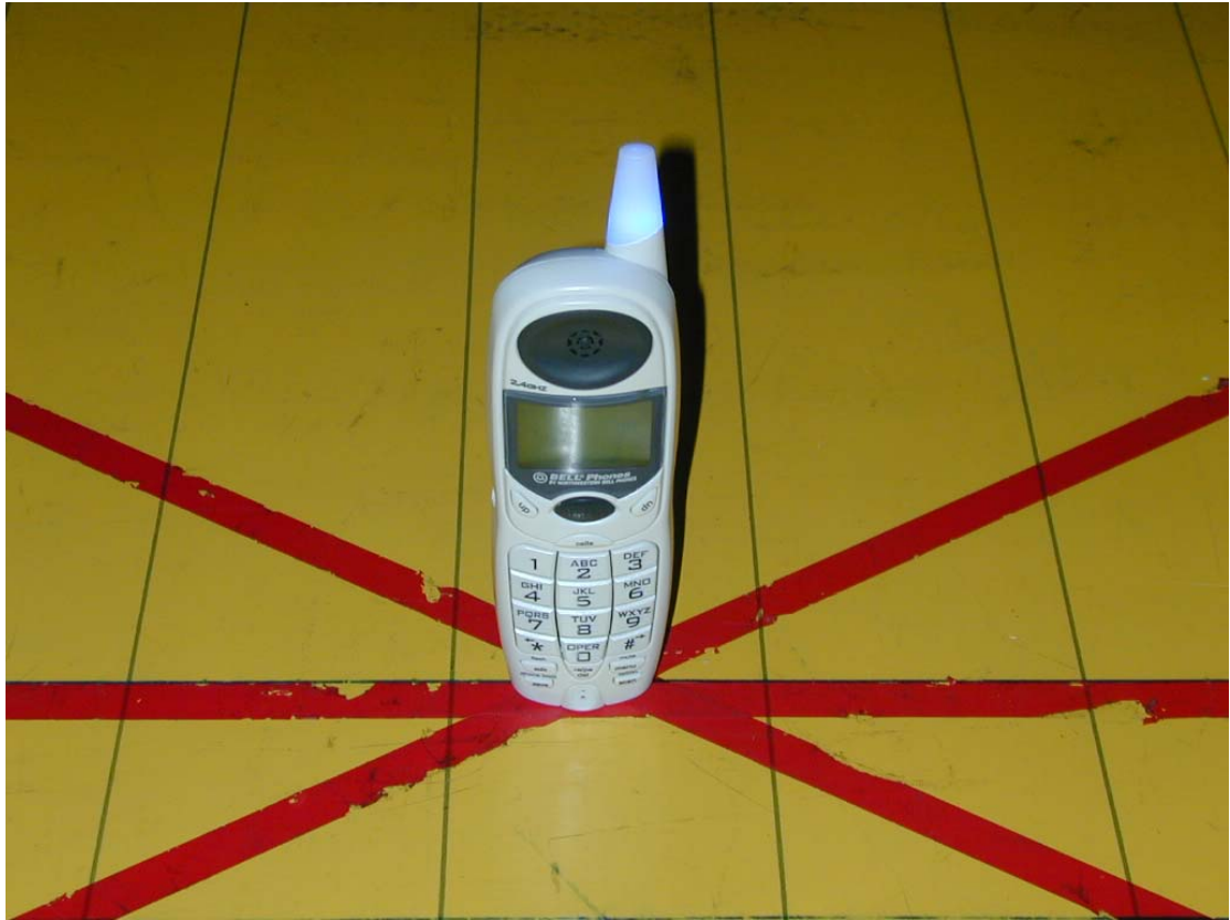
Photo 4: Radiated Emission Test Set-up photo (Handset)
