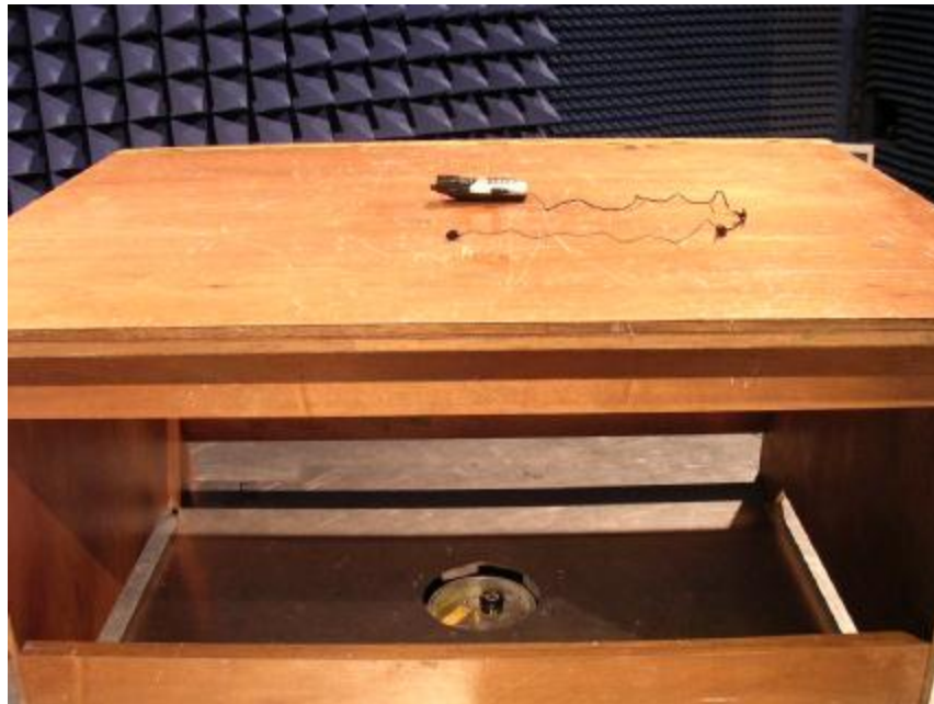
Photo 2: Radiated Emission Test Set-up (Handset)
