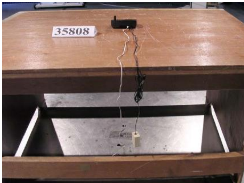
Photo 2: Radiated Emission Test Set-up (Base)
