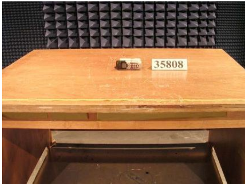
Photo 4: Radiated Emission Test Set-up (Handset)
