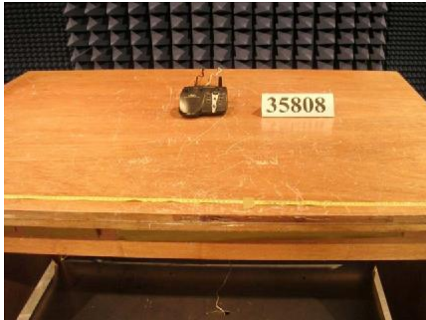
Photo 2: Radiated Emission Test Set-up (Base)
