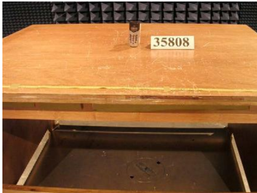
Photo 4: Radiated Emission Test Set-up (Handset)
