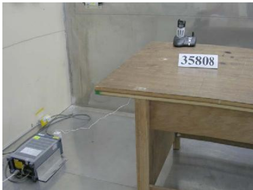
Photo 2: Conducted Emission Test Set-up
