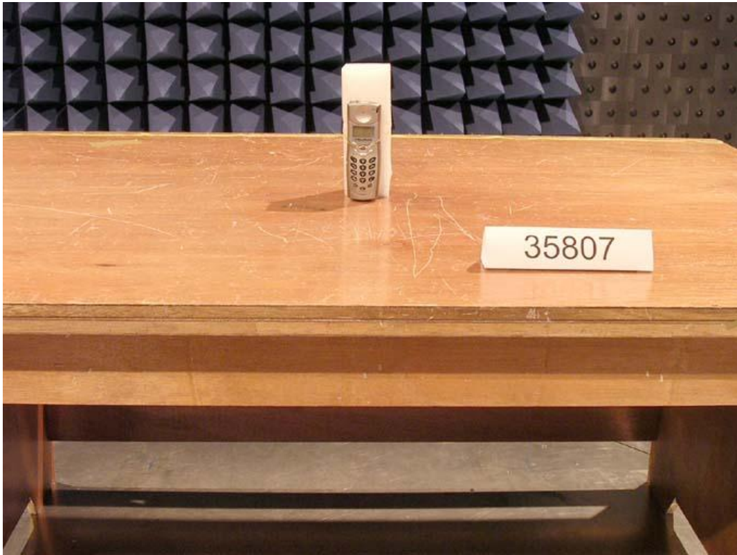
Photo 4: Radiated Emission Test Set-up (Handset)
