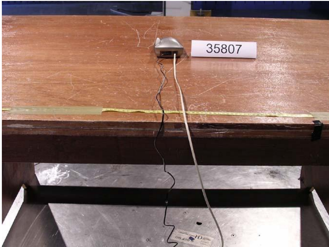
Photo 2: Radiated Emission Test Set-up (Base)
