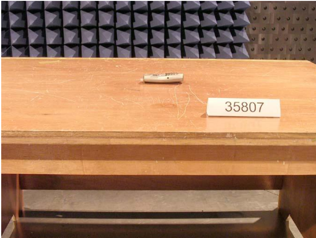
Photo 5: Radiated Emission Test Set-up (Handset)
