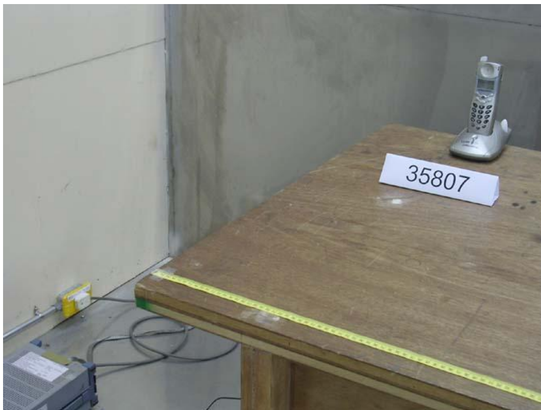
Photo 1: Conducted Emission Test Set-up
