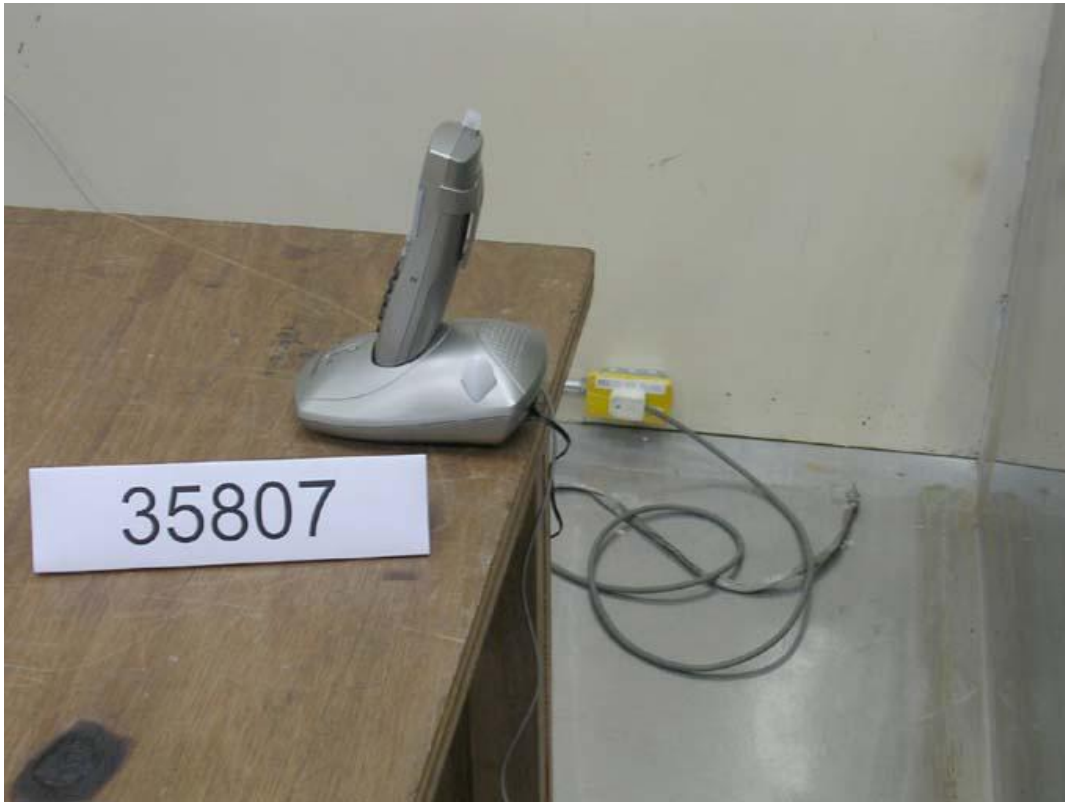
Photo 2: Conducted Emission Test Set-up
