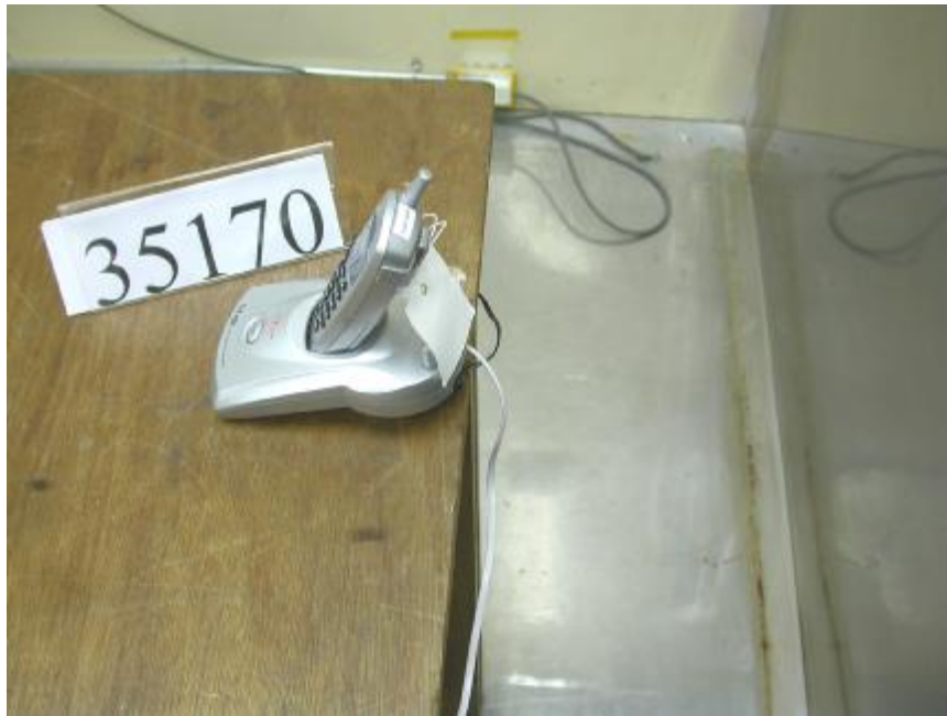
Photo 3: Conducted Emission Test Set-up
