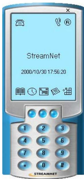
Each button of Keypad has the same function as Gz Phone Dial button of allotted number. Left two buttons of three buttons located on keypad have the same functions as Redial/Send buttons in the lower part of the phone. Right button is a Hang up button and if you click it with mouse, you can finish the call.
