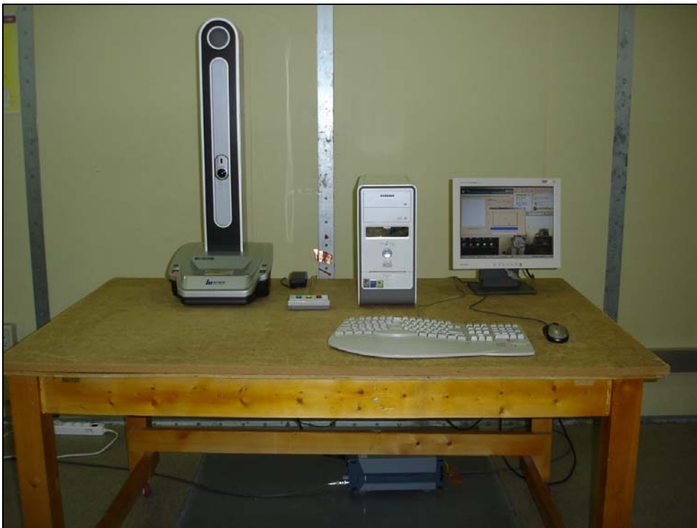
Photograph 1: Setup for Conducted Emissions
