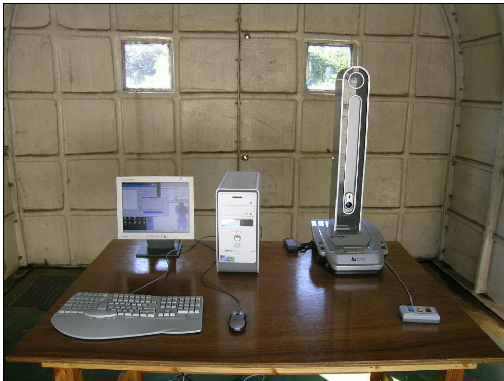
Photograph 2: Setup for Radiated Emissions
