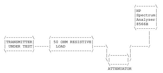
NAME OF TEST: SPURIOUS EMISSIONS AT ANTENNA TERMINALS
