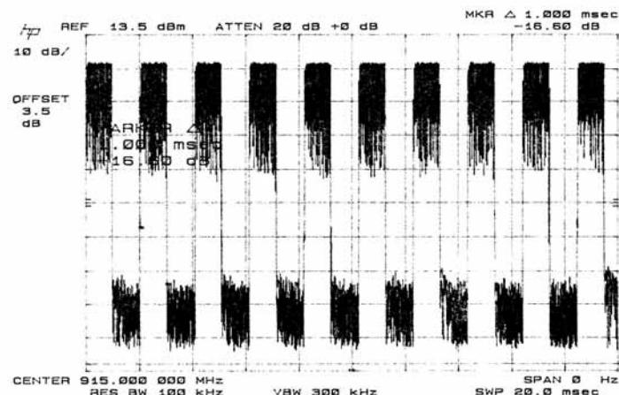
Duty cycle value =  $20\log(T\text{width}/T\text{period}) = 20\log(1*10^{-3}/2.040*10^{-3}) = -6.196$
