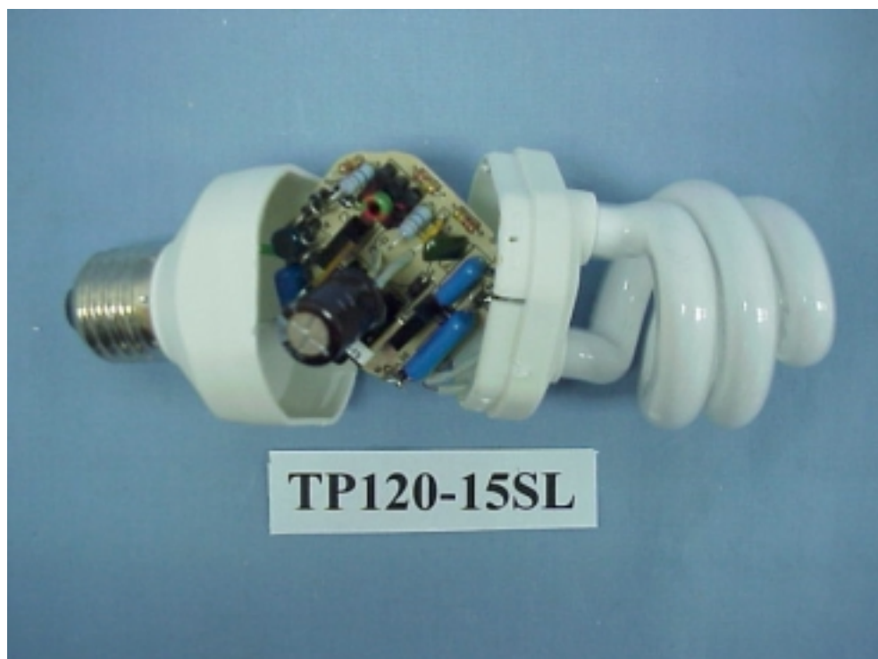
Figure 8 Compact Fluorescent Lamp (M/N: TP120-15SL) Cover Removed
