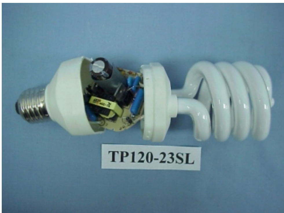
Figure 12 Compact Fluorescent Lamp (M/N: TP120-23SL) Cover Removed
