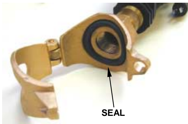
Figure 2-8. Apply Vaseline to Seal
