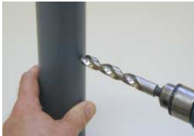
Figure 2-7. Drilling Pool Pipe
