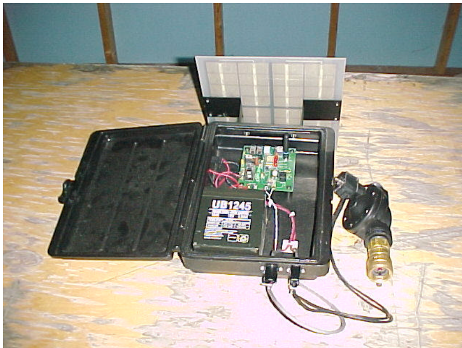
Figure 2 – View of Receiver Board mounted in case with solar panel
