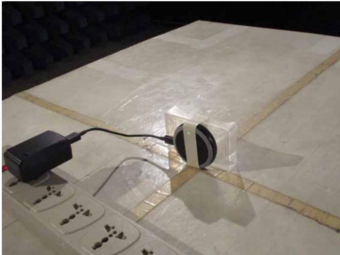
**RADIATED RF MEASUREMENT SETUP(Above 1G)**
