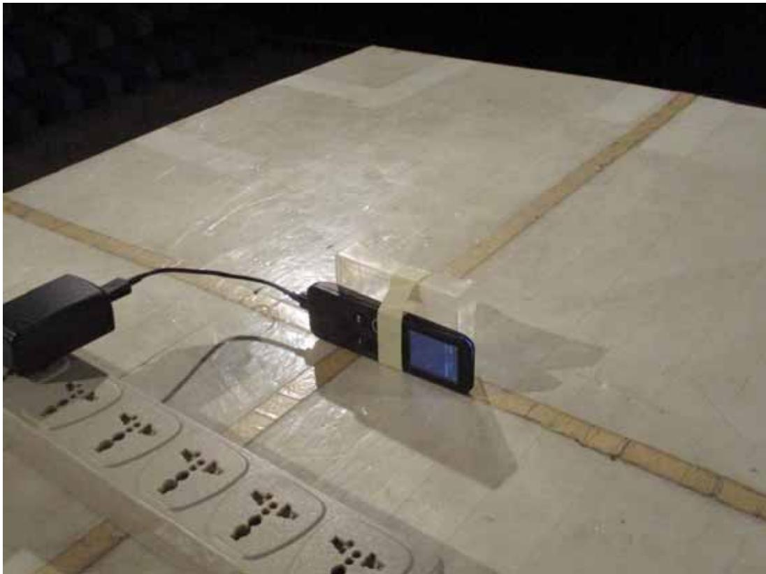
**RADIATED RF MEASUREMENT SETUP(Above 1G)**
