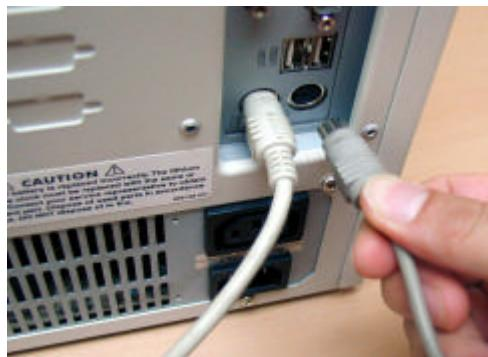
④ Connect PS/2 Connector with Mouse Connector
