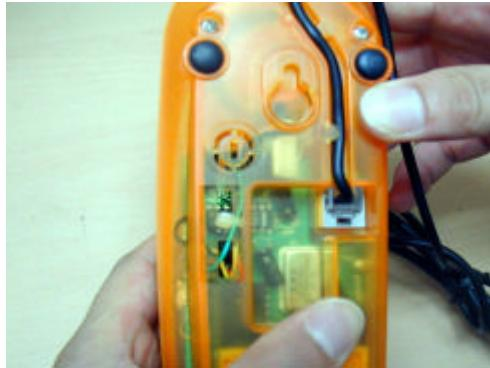
② Connect Serial Connector in COM1 Port
