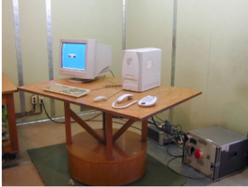
LINE CONDUCTED SETUP PHOTOGRAPH - FRONT VIEW
