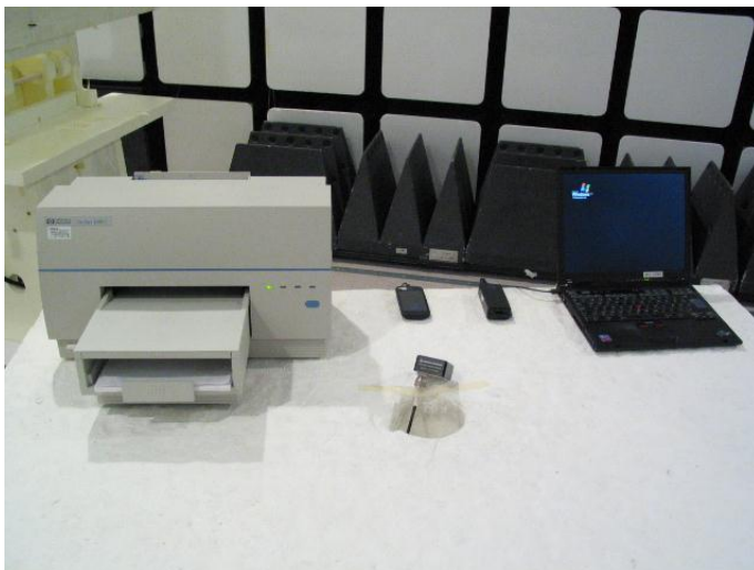
Picture 2. FCC Part 15B Radiated emissions
