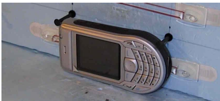
Picture 7: EUT in horizontal 2 (H2) orientation
