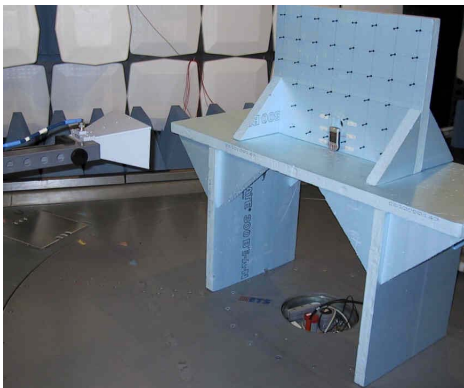
Picture 4: Radiated spurious emission measurement set-up for above 3 GHz measurements, EUT in vertical (V) orientation
