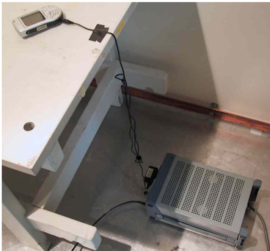
Picture 2: AC-power line conducted emissions test setup
