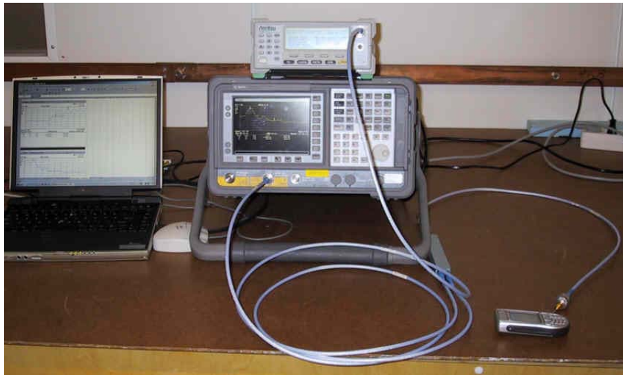
Picture 1: test set-up for conducted measurements from antenna port
