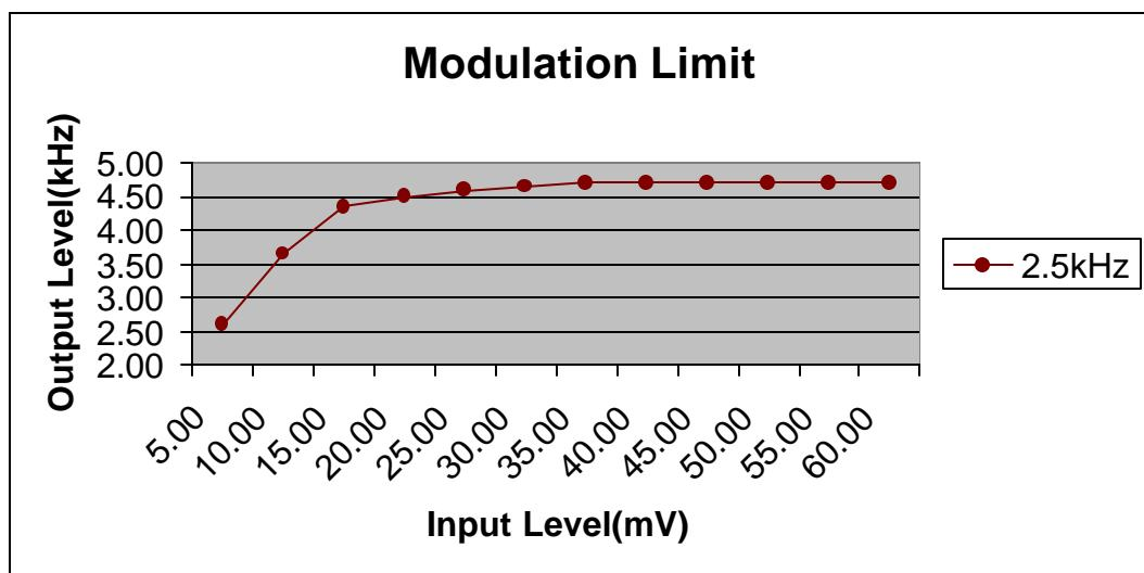
d) The conducted emission was tested with 2.5kHz modulation input
