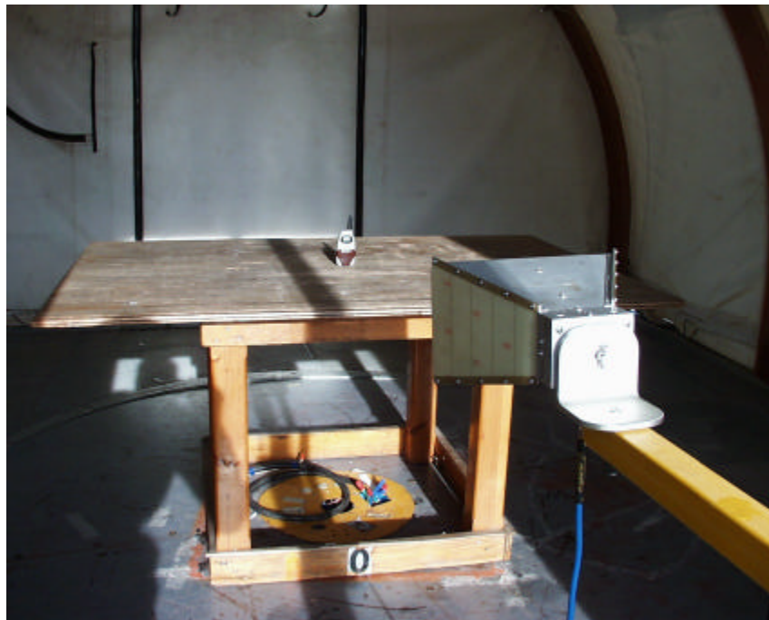
Radiated Emission above 1 GHz measurement setup
