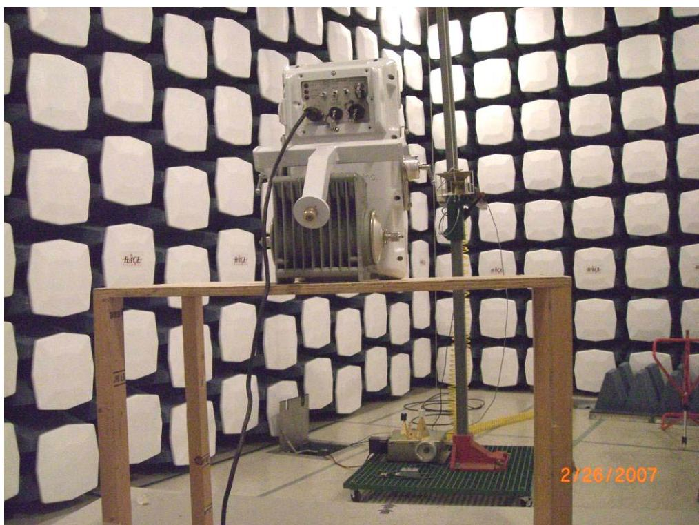
**Radiated Emissions – Rear View (18 – 26.5 GHz)**
