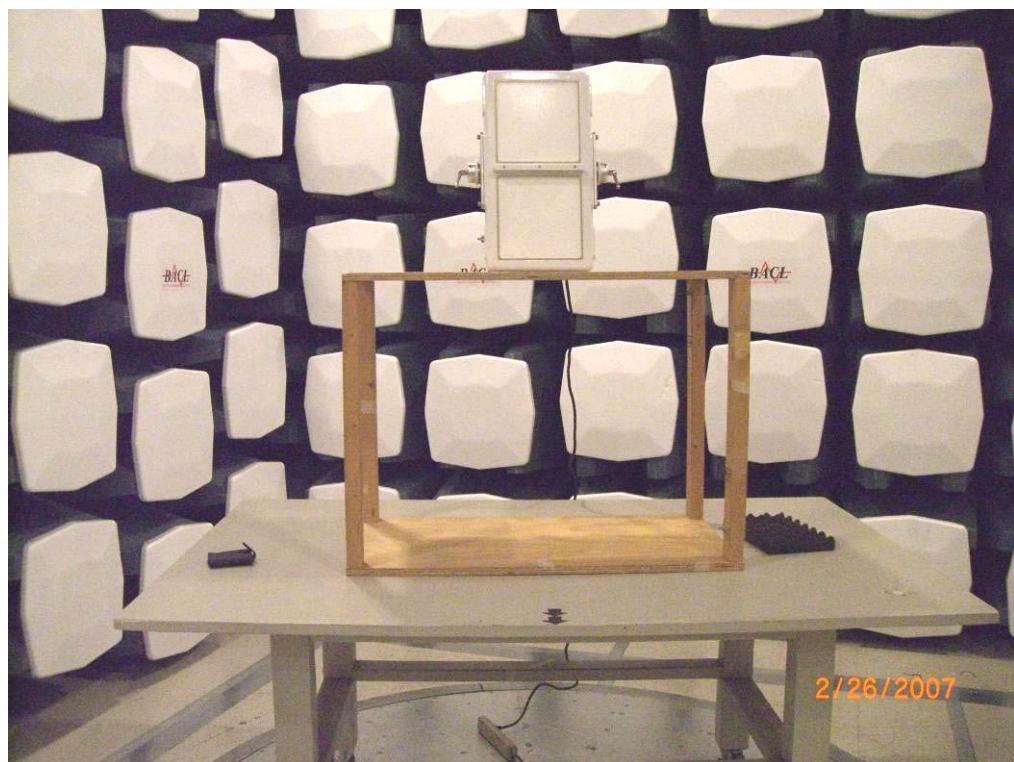
**Radiated Emissions – Rear View (1 – 18 GHz)\***
