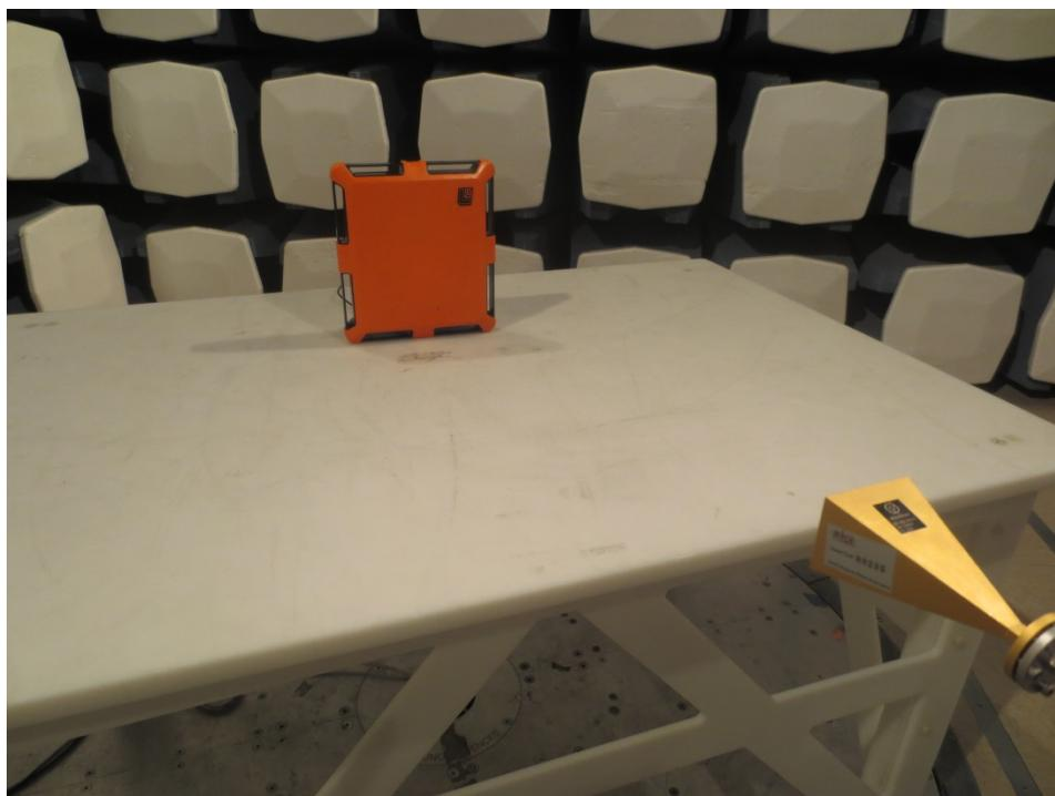
**10.11 Radiated Emission from 60 GHz to 90 GHz Rear View**
