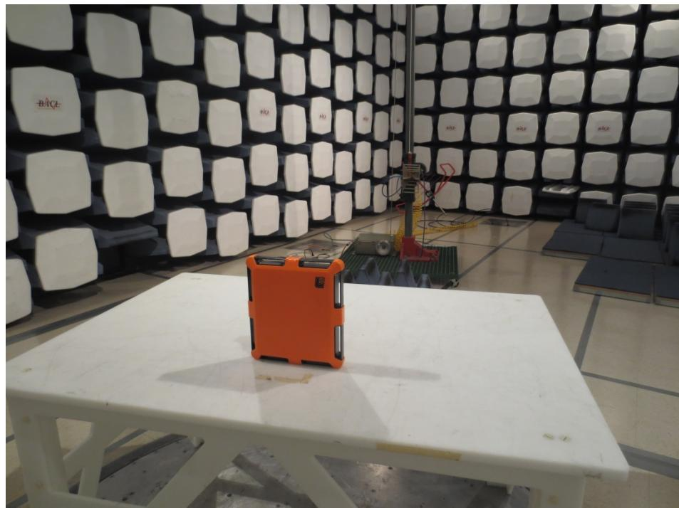
**10.4 Radiated Emission from 1 GHz to 18 GHz Front View**
