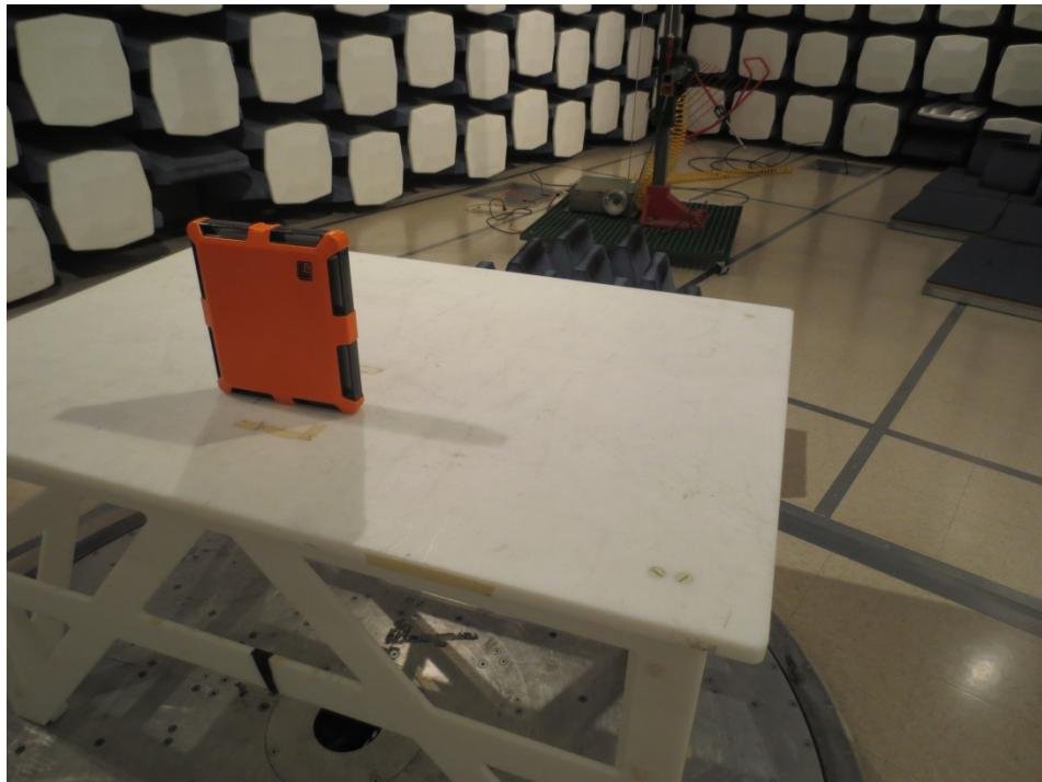
**10.8 Radiated Emission from 26 GHz to 40 GHz Front View**
