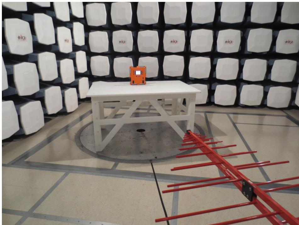
**10.3 Radiated Emission from 1 GHz to 18 GHz Rear View**
