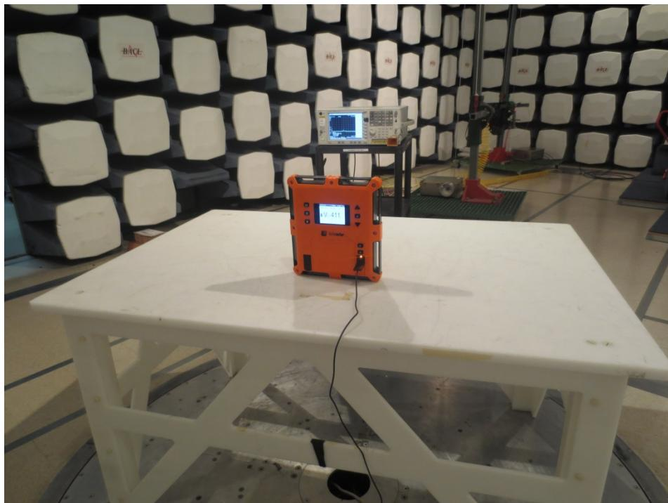
**10.10 Radiated Emission from 40 GHz to 60 GHz Front View**
