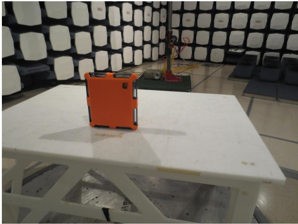
**10.6 Radiated Emission from 18 GHz to 26 GHz Front View**
