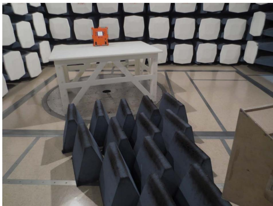
**10.5 Radiated Emission from 18 GHz to 26 GHz Rear View**
