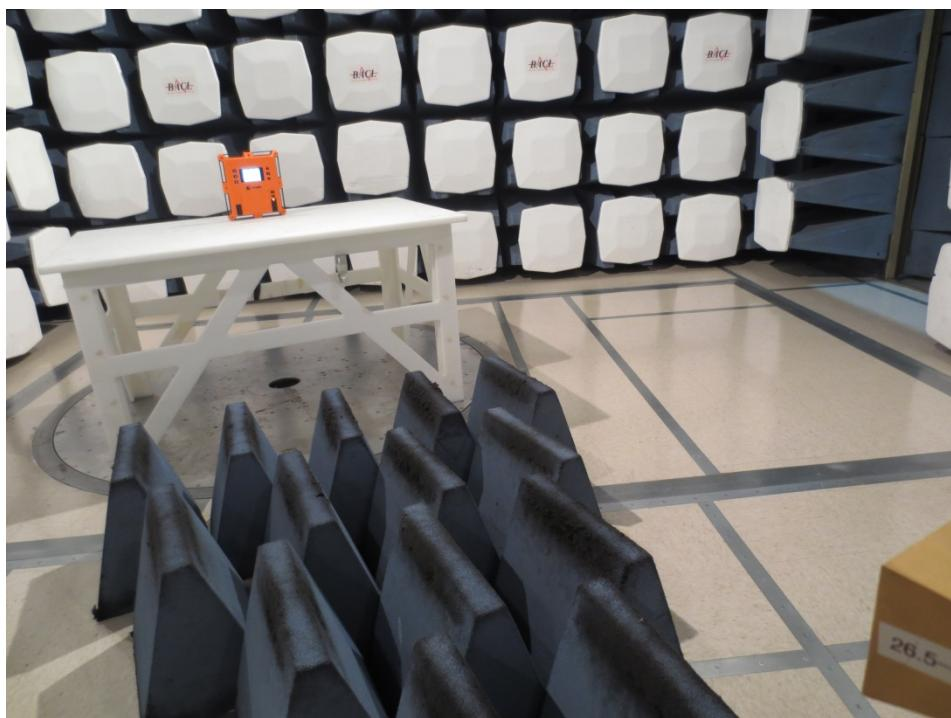
**10.9 Radiated Emission from 40 GHz to 60 GHz Rear View**
