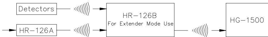
**‘Extender’ switch** – HR-126B is only transmitting the signal of Extender (HR-126A) not of the detector to HG-1500.
