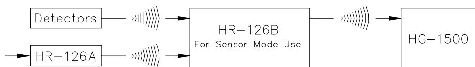
‘Sensor’ switch – HR-126B is only transmitting the signal of the detector not of Extender (HR-126A ) to HG-1500.
