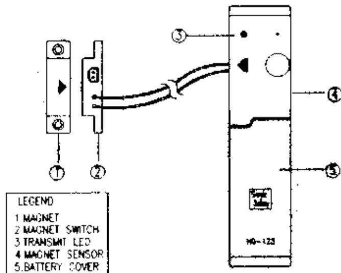
.HG-122 is a door/window detector with 12V alkaline battery.
