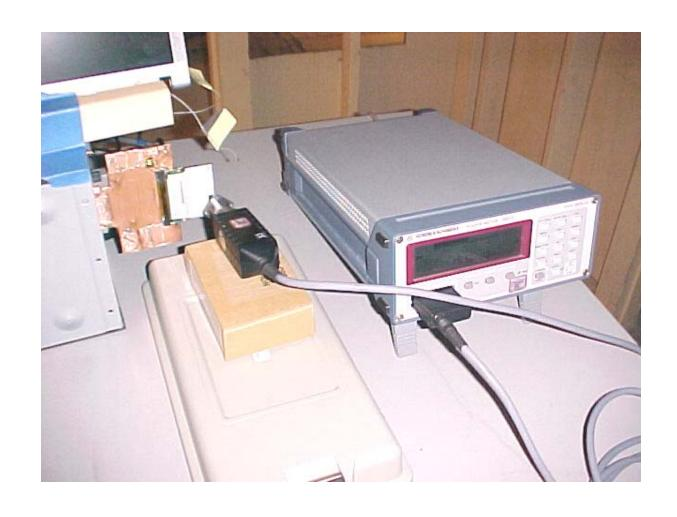
Maximum Peak Output Power Measurement Setup
