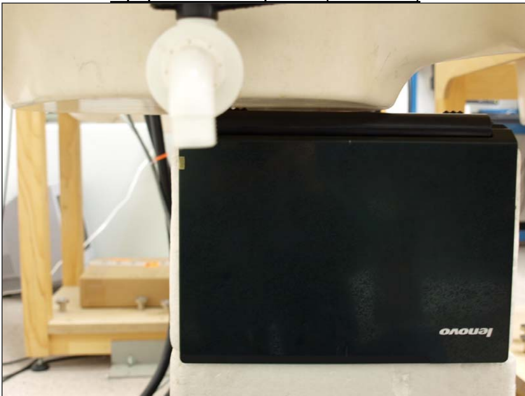
Laptop Mode with SAM phantom (2.4 GHz band)
