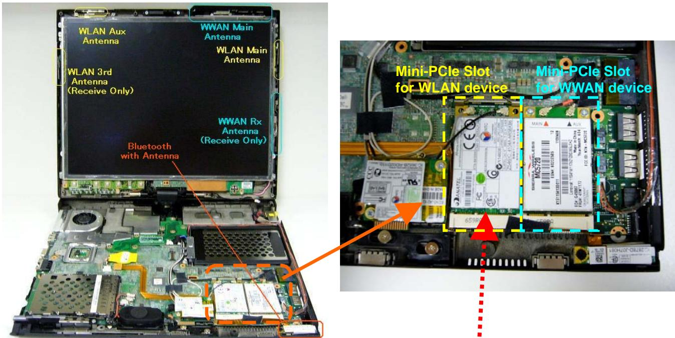
The certification label is stuck on the top side of the applying transmitter device, and the FCC ID is visible when the palm rest assembly is removed.
