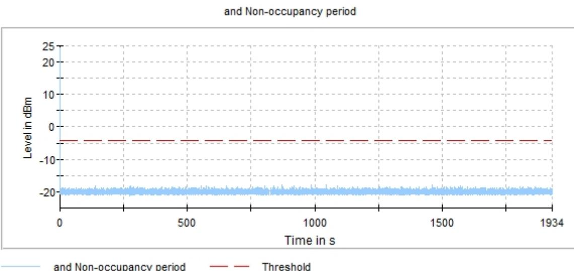
**No transmission of any type has occurred for 30 minutes, test PASS**
