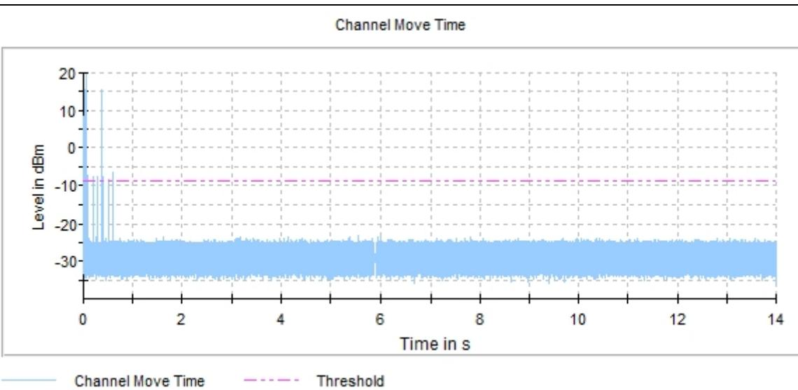
**Channel move time < 10s, test PASS**
