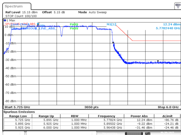
BE-NR-HIGH-PEAK, SISO-B, 802.11ac160-VHT0, Ch163
