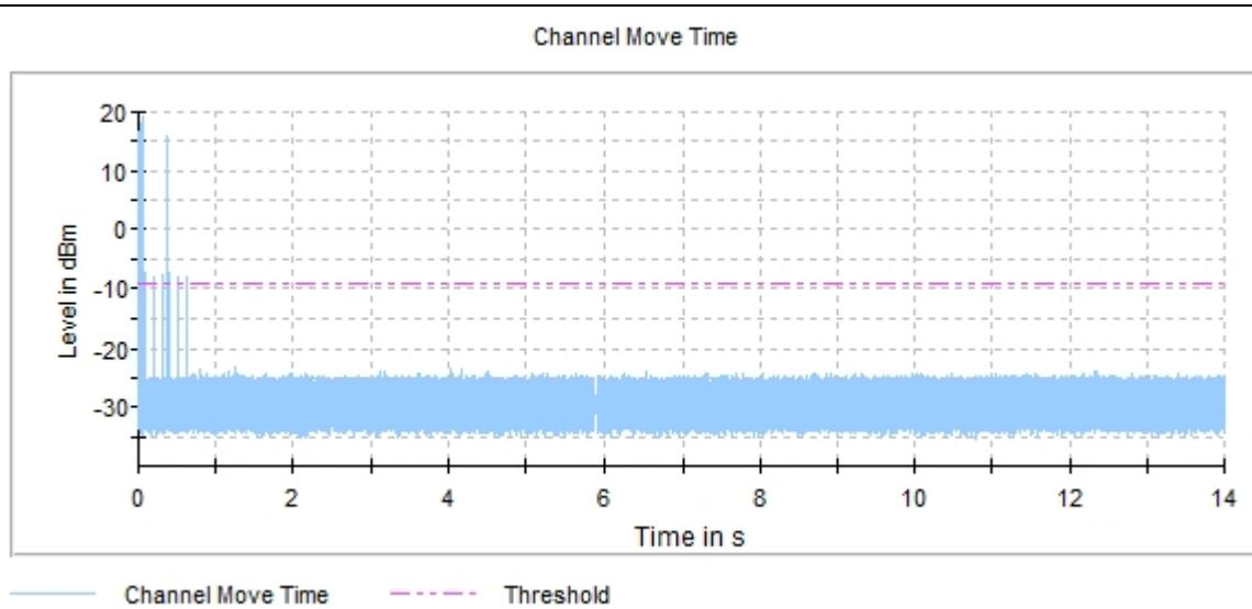
**Channel move time < 10s, test PASS**
